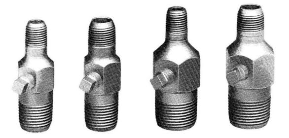
Eclipse Flame Scanner Adapters permit quick, easy installation of ultraviolet flame scanners to burner connections of a different pipe size. Made from heavy steel, these adapters are supplied with a 1/8" N.P.T. tap to permit connection of a purge air line, if required.
